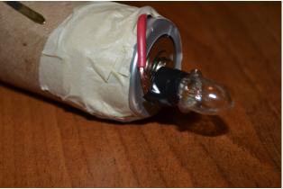
16. Securely tape the lightbulb holder onto the top of the flashlight. Don't be afraid to use a lot of tape! Double check that it is working by connecting the switch while you are taping it. You can also use an extra piece of cardboard to create a holder as well.
