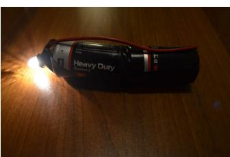
4. Tape the lightbulb to the positive end of the battery.
