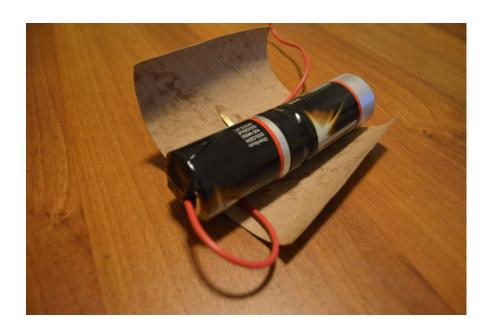
11. Tape the toilet paper or paper towel roll back together using masking tape or duct tape. Make sure that the end of the other wire is sticking out of the top of the tube on the same side as the positive end of the battery (with the bump).
